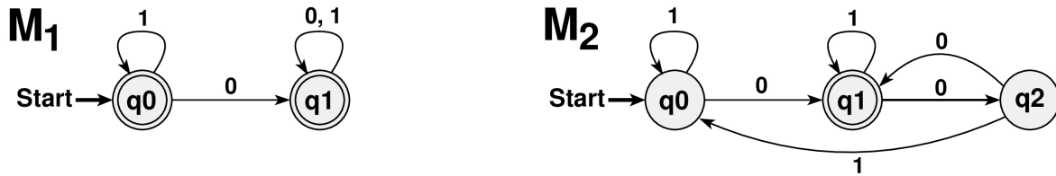
Fig. 2.16: Construct the automaton M_1 \times M_2 that accepts the intersection language L(M_1) \cap L(M_2)
